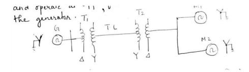
6. Obtain the impedance diagram of the electrical power system shown in figure. Mark all the impedance values in per unit on a base of 50MVA, 138kV in the  $40\Omega$  line.
