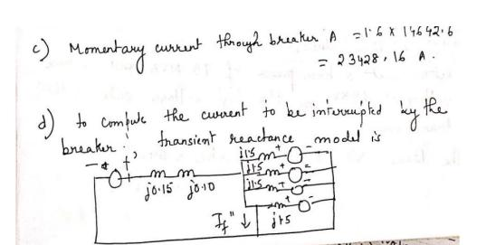
the coverent to be intrompted by the preaker A  $i_{p} = 3 \times \frac{1}{j_{1} \cdot 5} + \frac{1}{j_{0} \cdot 25} = -j_{6} p_{1} u_{2}$ To make the allowance for d.c offset covery 1.1 × 6×2091 = 13,805.88 A.
