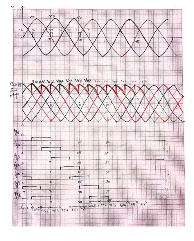
$$V_{0} = \frac{6}{2\pi} \int V_{AB} d\omega t$$
