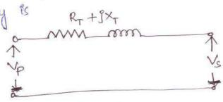
RT = per unit resistance XT = per unit reactance. By defination; Per unit reactance (XT) = Actual Reactance (X) Actual reactance,  $X = X_T \cdot \begin{pmatrix} x \\ T \end{pmatrix}$
