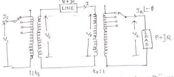
\* It is required to determine the tap-changing ratios required to completely compensate for the voltage drop in the line.
