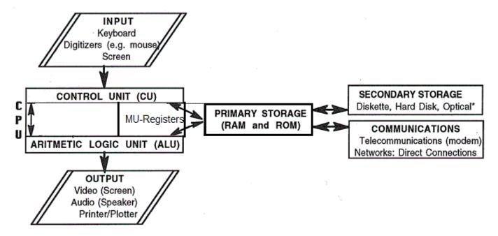
Input unit: The input unit that links the external environment to input data & tasks with the computer system to execute. Data are entered in different forms through different input devices. Keyboard is used for characters input. Mouse is used in GUI (Graphic User Interface). Internally data is processed in machine readable form.
