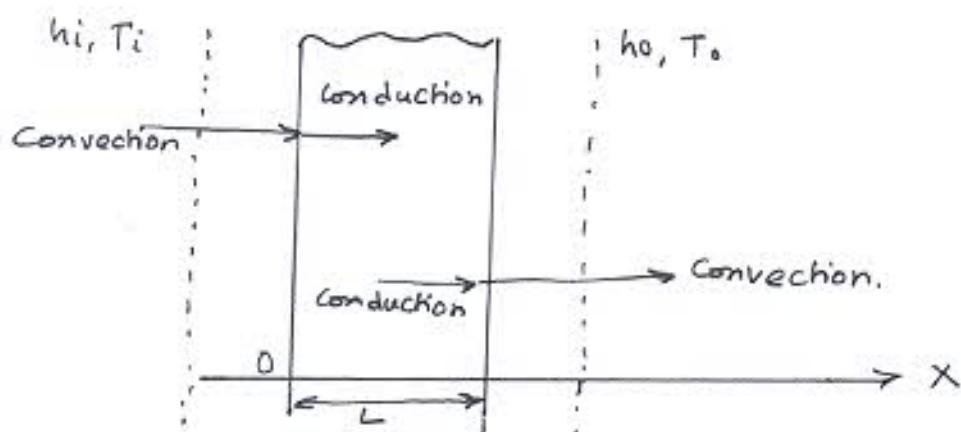
$$\text{At } n=0, h_i [T_i - T(0,t)] = -k \left( \frac{\partial T}{\partial x} \right)(0,t)$$
