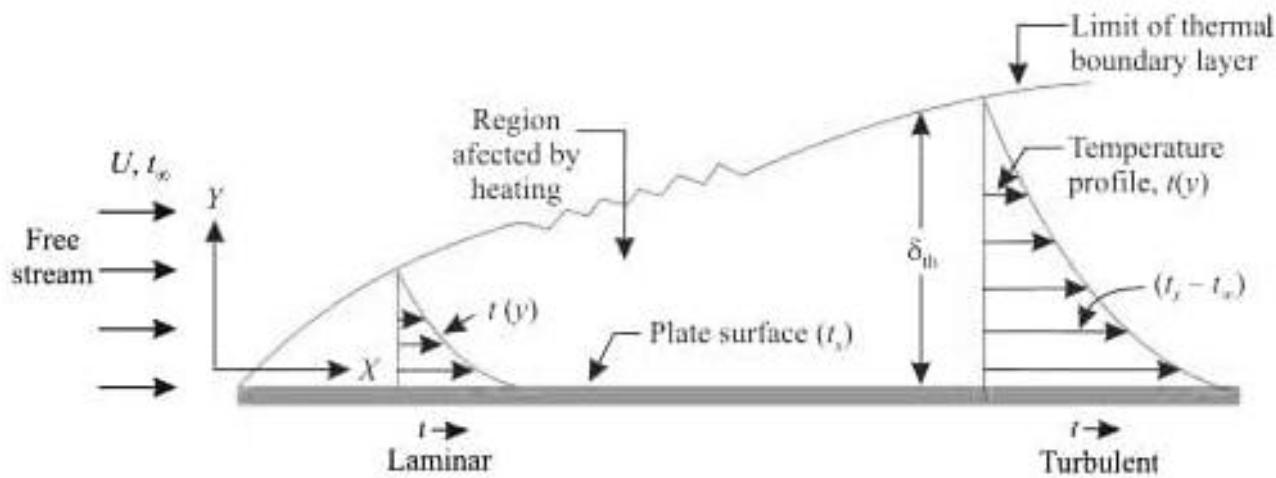
Whenever flow of fluid takes place past a heated or cold surface, a temperature field is set up in the vicinity of the surface. If the surface is hotter than the fluid, the temperature distribution will be shown as in the above fig. The zone over this layer wherein the temperature field exists is called as thermal boundary layer.
