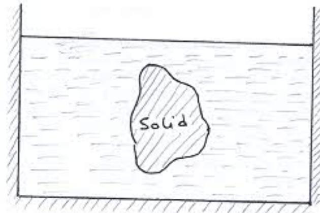
Consider a solid suddenly immersed in a well stirred fluid maintained at a uniform temp  $T_\infty$ .
