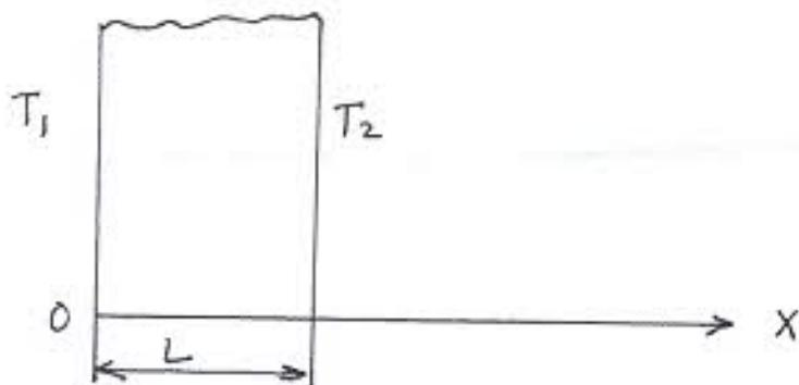
The specified temperature can be constant (steady state heat conduction) or may vary with time.
