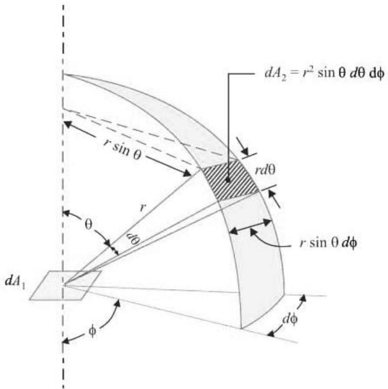
The fig shows a small black surface of area  $dA$ , emitting radiations in different directions. A black body radiation collector through which the radiation passes is located at an angular position characterised by zenith angle  $\theta$  towards the surface normal & angle  $\phi$  of a spherical co-ordinate system. The collector subtends a solid angle  $d\omega$  when viewed from a point on the emitter.
