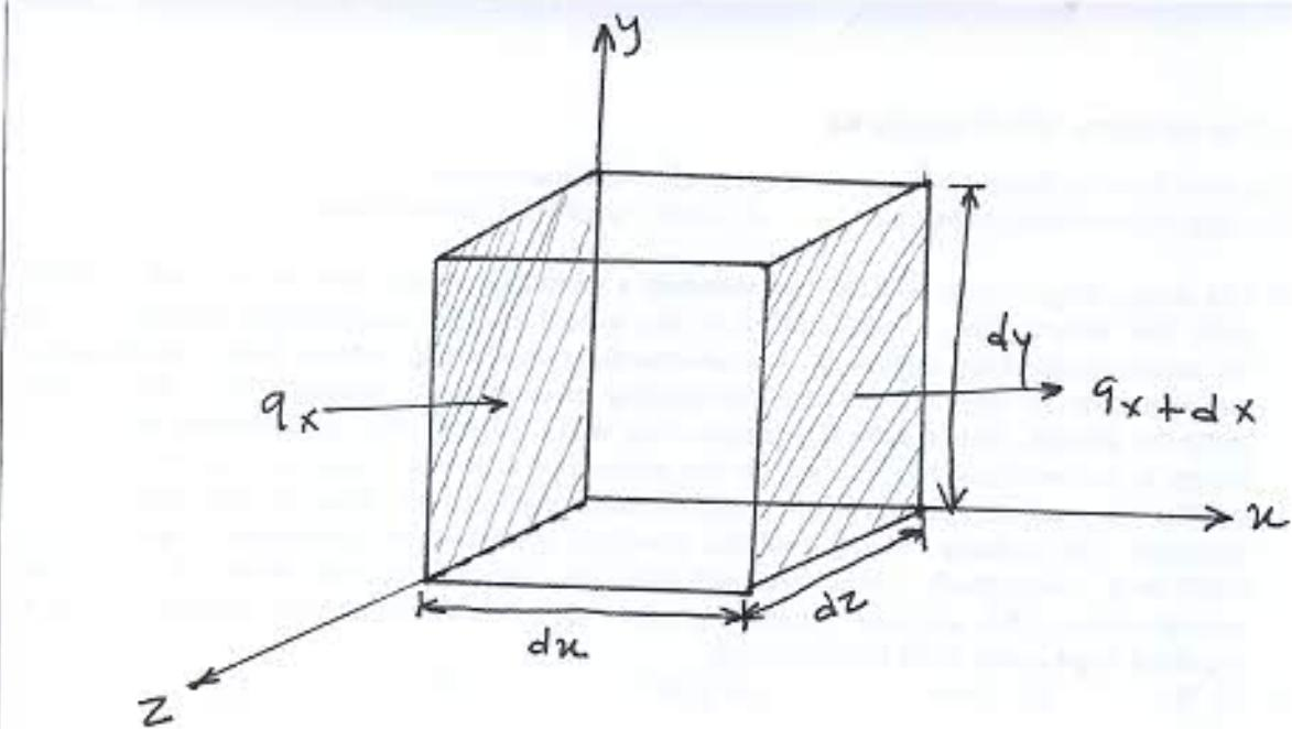
Consider a small rectangular element of dimensions  $dx, dy$  &  $dz$  in  $x, y$  &  $z$  directions respectively.
