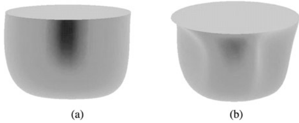
Fig. 6.5 Influence of local manipulation of the derivative curve on the shape of the surface
