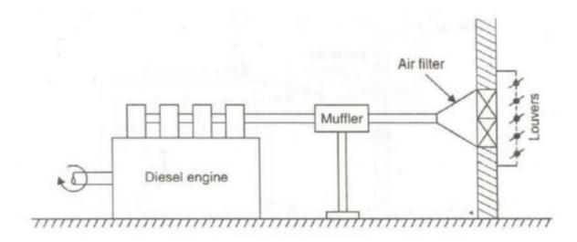
Following precautions should be taken while constructing a suitable air intake system:
