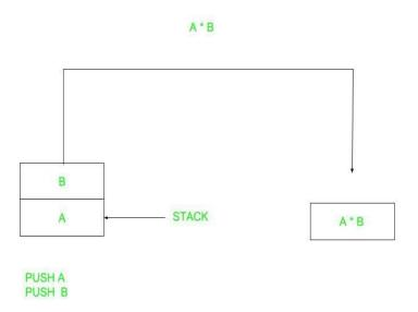
A stack based computer do not use address field in instruction. To evaluate a expression first it is converted to revere Polish Notation i.e. Post fix Notation.
