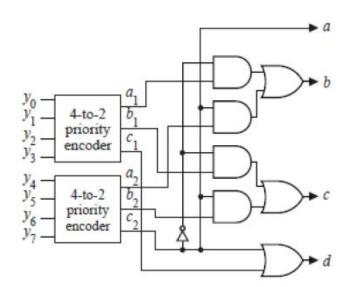
If any of the inputs  $y_0$  through  $y_\gamma$  is 1, then d of the 8-to-3 decoder should be 1. But in that case,  $c_1$  or  $c_2$  of one of the 4-to-2 decoders will be 1. So  $d = c_1 + c_2$ .
