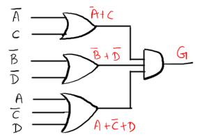
The hazard-free expression for G is (A'+C) (B'+D') (A+C'+D) (A+B'+C'). Its OR-AND circuit diagram is shown below.
