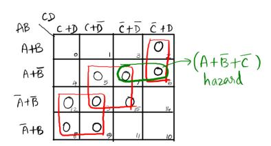
The hazard is caused by maxterms M6 & M7. It is a Static-0-hazard. The term corresponding to the hazard is (A+B'+C').
