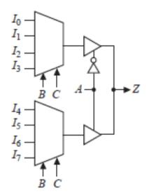
An 8:1 MUX requires 8 inputs (I0, I1, I2, I3, I4, I5, I6 and I7), 3 select lines (A, B, C) and 1 output Z.
