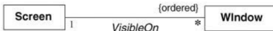
Figure 3.15 Ordering the objects for an association end. Ordering sometimes occurs for “many” multiplicity.
