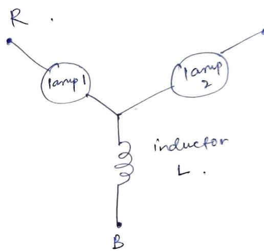
The static phase sequence indicator consists of two lamps and an indicator. The device whose phase sequence is to be determined is connected to the static phase sequence indicators. If the lamp 1 is dim and lamp 2 glows brightly, then the phase sequence of supply is RYB.
