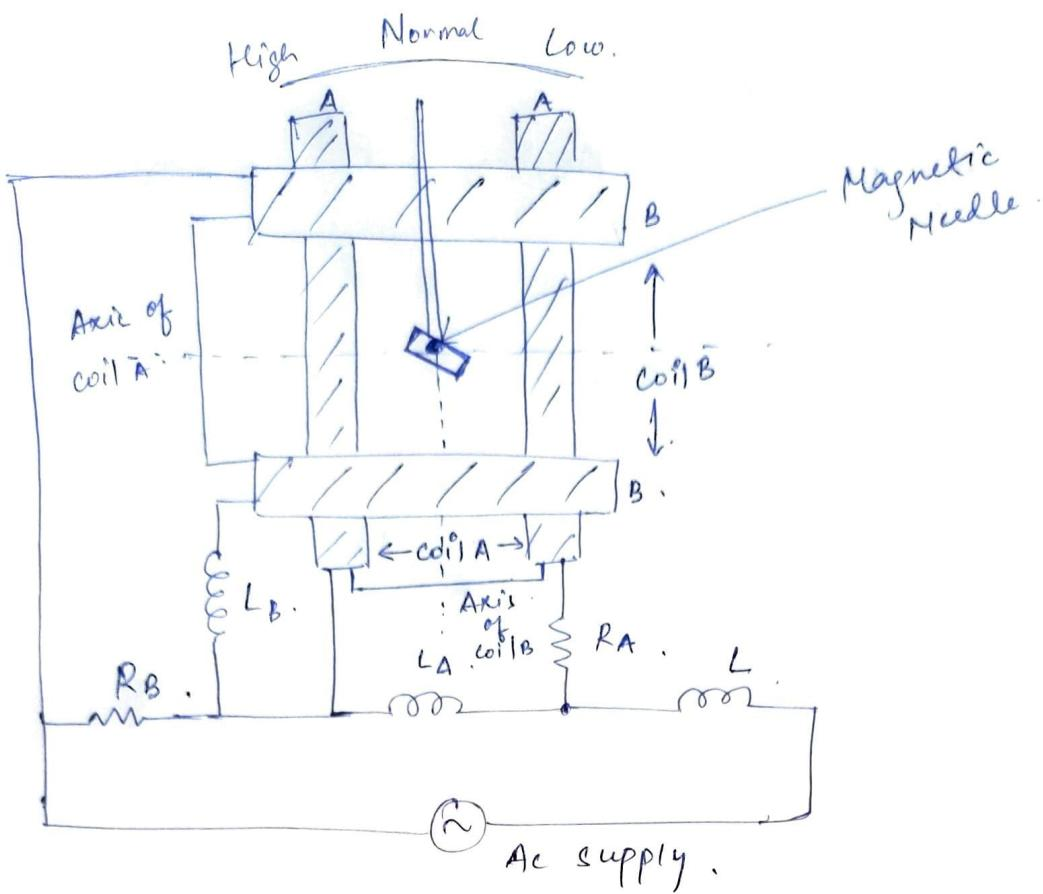
Principle  $\rightarrow$  When an current flows through the two coils, which are perpendicular to each other, due to these currents some magnetic field will produce & thus the magnetic needle will deflect towards the stronger magnetic field showing the measurements of frequency in the meter.
