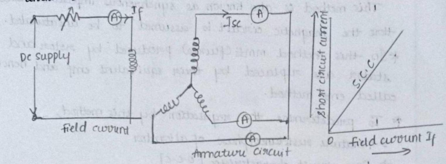
\* The open-circuit voltage coronesponding to field current If is Eq. the s.c armatrone current corresponding to field covurnt If is I,
