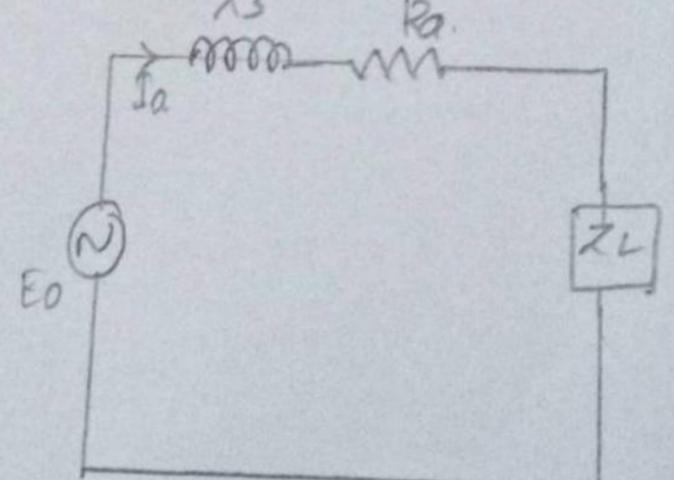
\* The synchronous neactance is a quictitions neactance employed to account for voltage effects in armature
