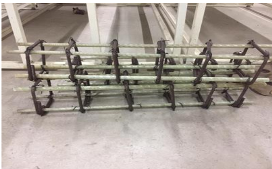
Fig 5.2 GFRP reinforcement (left) and steel reinforcement (right)
