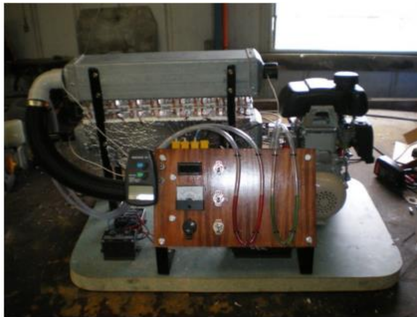
Fig. 15. An exhaust heat recovery system using heat pipes to transfer heat both to and from the TEGs.
