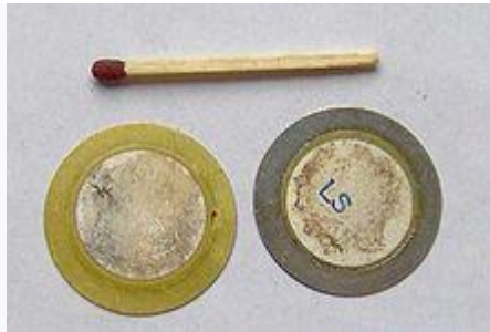
Metal disks with piezo material, used in buzzers or as contact microphones
