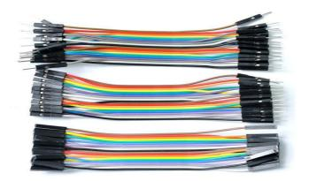
A jump wire (also known as jumper wire, or jumper) is an electrical wire, or group of them in a cable, with a connector or pin at each end (or sometimes without them – simply "tinned"), which is normally used to interconnect the components of a breadboard or other prototype or test circuit, internally or with other equipment or components, without soldering.<sup>[1]</sup>
