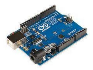
Arduino Uno is a microcontroller board based on the ATmega328P ( datasheet). It has
