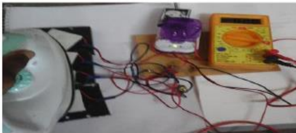
Figure 5.1: Charging the sample mobile battery using TEG by waste heat.
