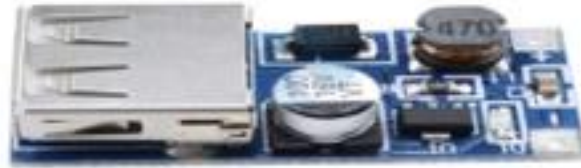
Figure 3.3: DC-DC power boost module.
