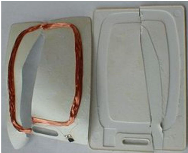
Figure RFID Card showing the Microchip and Antenna
