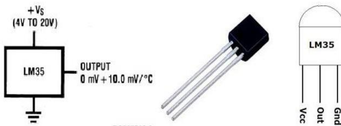
Figure 3.3.1 LM35 Temperature sensor schematic and ports
