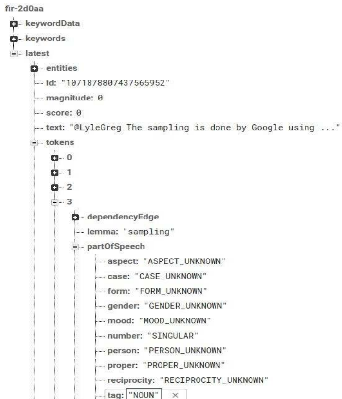
Figure5.1.1 Example of the Firebase database in our example application. The child-node 'latest' indicates the last tweet that was analyzed by the Google NLP service.
