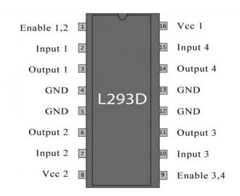
A motor driver IC is an integrated circuit chip which is usually used to control motors in autonomous robots. Motor driver ICs act as an interface between microprocessors in robots and the motors in the robot. The most commonly used motor driver IC's are from the L293 series such as L293D, L293NE, etc. These ICs are designed to control 2 DC
