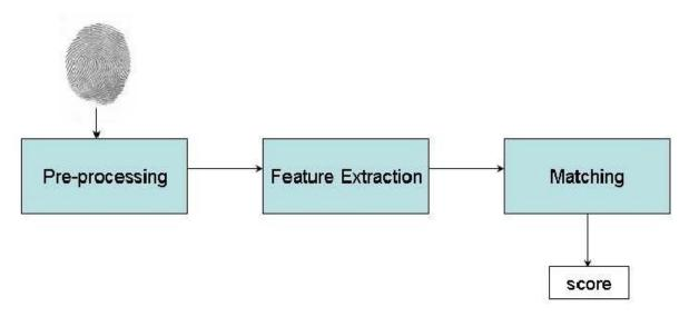
The main modules of a fingerprint verification system are:
