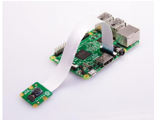
Fig 26 Connection of Raspberry Pi camera to Raspberry Pi
