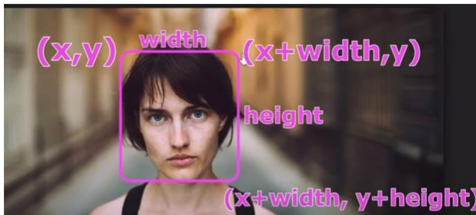
Figure 18. Defining a window for face detection
