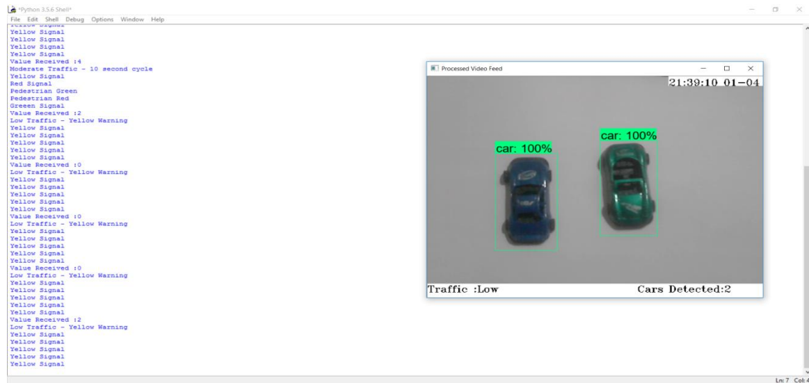
Fig 7.1 Traffic signal cycle in a low traffic condition.
