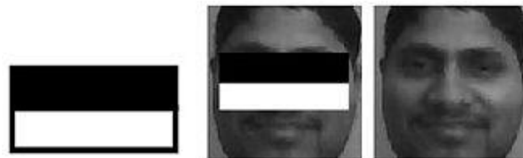
Figure 3.3 Haar Feature that looks similar to the eye region which is darker than the upper cheeks is applied onto a face
