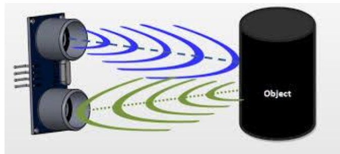
Fig 1.5.2 : Working of US sensor
