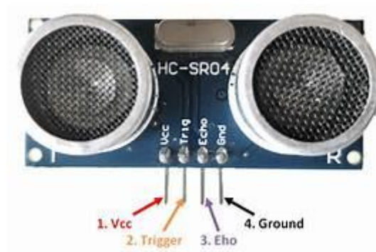
Fig 3.3.4 : Pin diagram of US sensor
