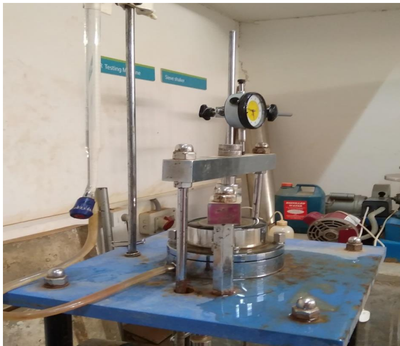
Fig 6.2(a):- Consolidation setup wherein pressure of 0.01kg/cm 2 is applied.
