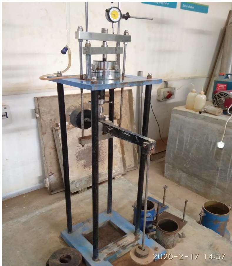
Fig 6.2(a):- Consolidation setup wherein pressure of 0.01kg/cm 2 is applied.
