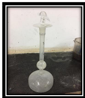
Fig 4.2.2.3 (b) Le- Chatelier's apparatus
