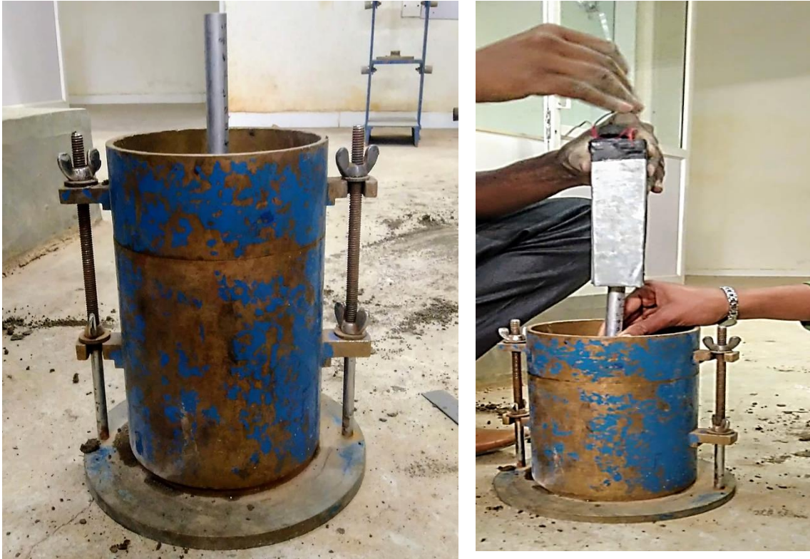
Fig: 1 and Fig: 2 Small scale experiment using open-driven piles in CBR mould.
