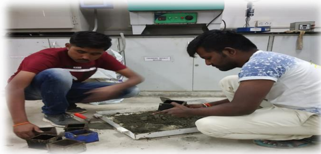
Figure 4. 9- Casting of cubes
