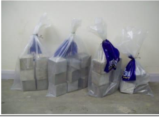
Fig. 2.5 Test cubes under summer curing environment
