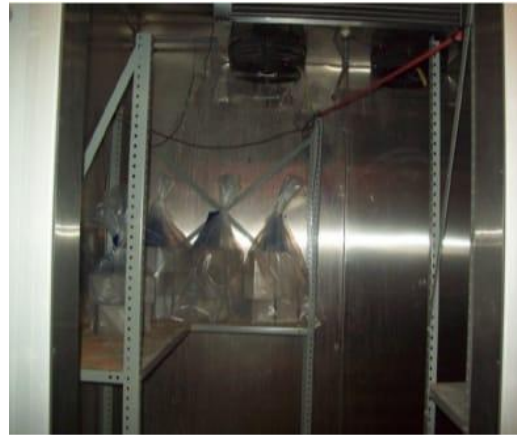
Fig 2.7 Test cubes under winter curing environment
