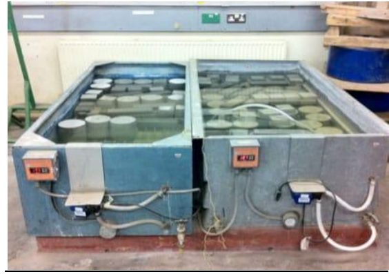
Fig. 2.6 Test cubes under water curing environment
