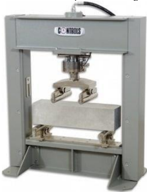
Fig.4: Flexural Test Machine and Concrete Specimen Applications of Flexural Test on Concrete
