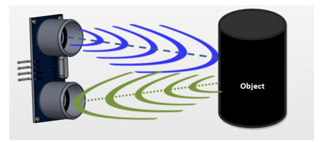
Now, to calculate the distance using the above formulae, we should know the Speed and time. Since we are using the Ultrasonic wave we know the universal speed of US wave at room conditions which is 330m/s. The circuitry inbuilt on the module will calculate the time taken for the US wave to come back and turns on the echo pin high for that same particular amount of time, this way we can also know the time taken. Now simply calculate the distance using a microcontroller or microprocessor.
