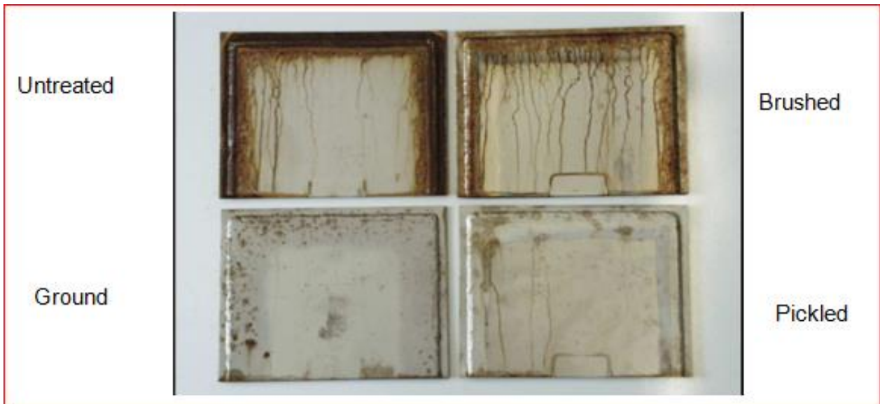
Figure. 6.8: Effect of heat tint colors and weld cleaning operations on the salt spray test resistance of stainless steel 1.4301
