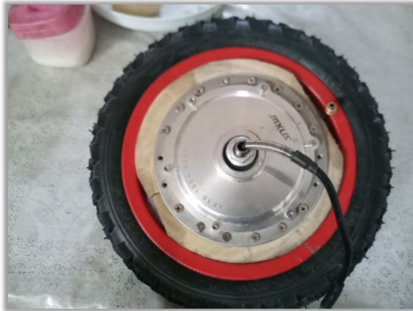
Fig 4.7 : Hub motor attached to wheel
