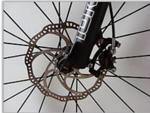
Fig 3.9 : Disc brake in a cycle
