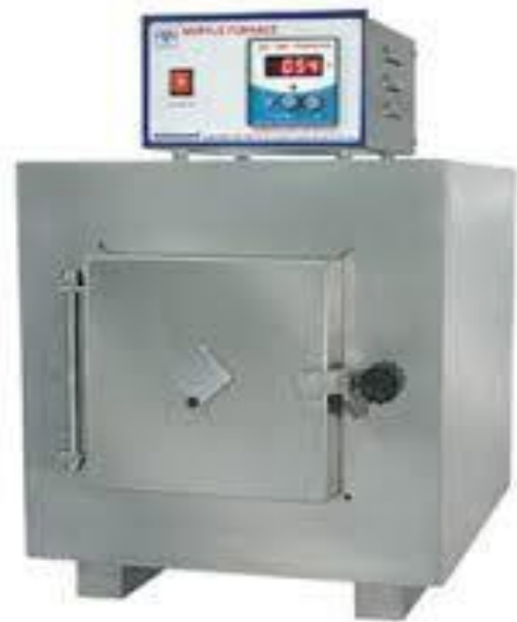
Fig :3.2. Muffle Furnace
