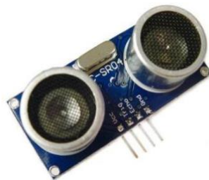
Fig.3.13 Adraxx HC-SR04 Ultrasonic/Sonar Distance Measuring Sensor
