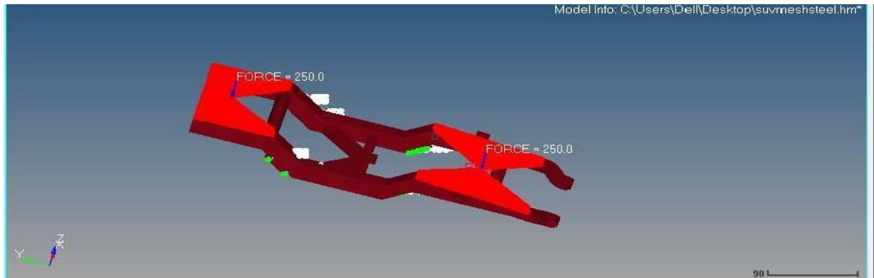
Fig 8.3 Meshed chassis with a boundary and loading condition
