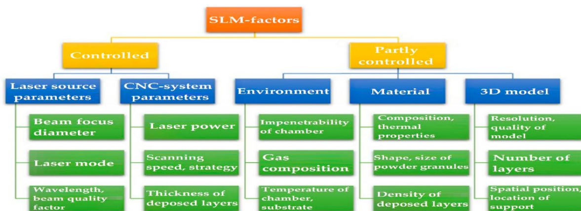
Figure 15: Input Parameters for the SLM process.
