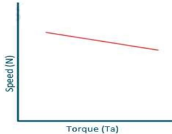
Fig 5.9: Speed Torque characteristics
