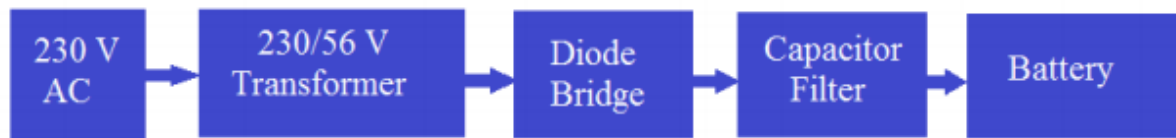
Fig. 5.2 Charging of Lead Acid Battery
