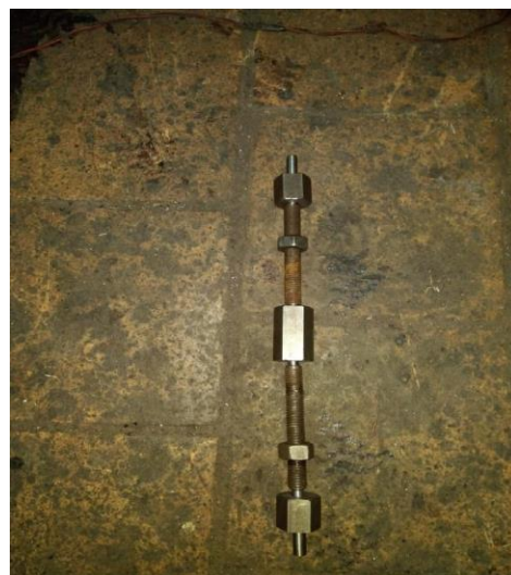
FIG 6.6 Lead Srew attached with screw & bolt
