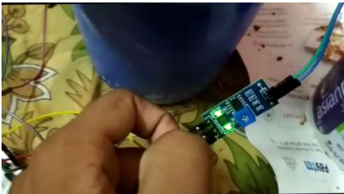
Fig 6.4 The moisture sensor's sensitivity is decided by the screw , if we tight it more, the sensitivity is increased and if we loosen it, the sensitivity is decreased.
