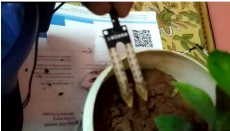
Fig 6.2 Then we take out the moisture sensor and now we see that the value of moisture becomes much lesser than threshold.
