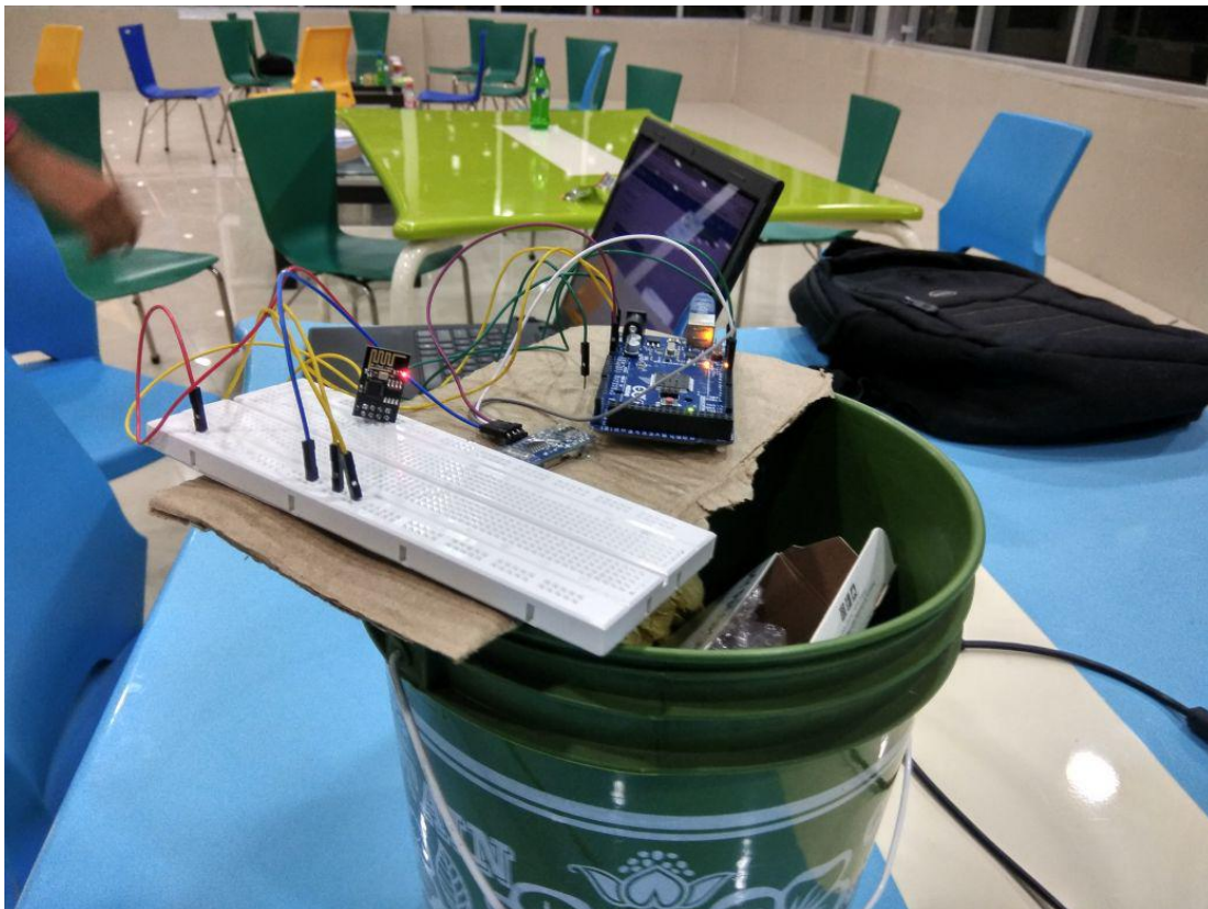
Fig 6.1 Shows that smart bin in which the UR Sensor is deployed to detect
