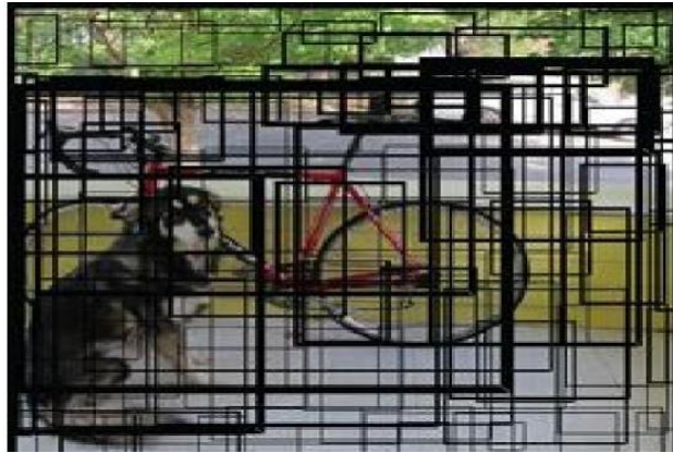
Fig. 8- Calculate Bounding Boxes and confidence score for each box.
