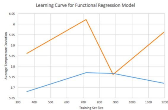
Fig. 2.3 The learning curve for the functional regression model, showing the rms error averaged across all seven days as a function of the training set size.
