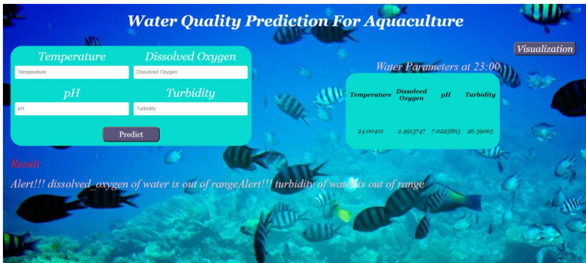
Figure 7.7 Alert Message when DO and Turbidity both are Out of Range
