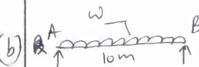
$R_A = R_B = \frac{10\omega}{2} = 5\omega$<br>$M_{max} = 5\omega \times 5 - 5\omega \left(\frac{5}{2}\right) = 12.5\omega \text{ N-m}$<br>$\sigma_{per} = \frac{60}{6} = 10 \text{ MPa} ; \omega = 5184 \frac{\text{N}}{\text{m}}$ | (2)<br>(2)<br>(6) |
