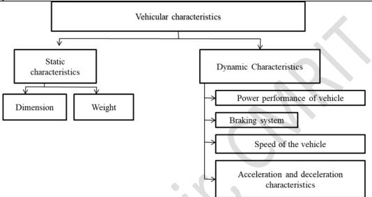
Static characteristics influencing high way design include dimensions and weight. Their affects on high way design are provided in the following table
