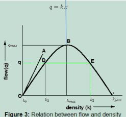
Similarly when the traffic flow is very less, no vehicle itself, hence speed will be less. As traffic flow increases, speed increases, and after a peak with more traffic flow, interaction between the vehicles increases and speed decreases. Along with traffic density increases and reaches jam density. This is presented in Fig. 2.
