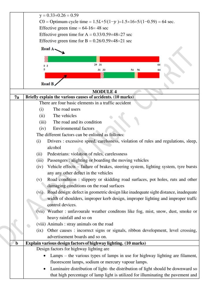
the adjacent areas. The distribution of luminaire should cover the pavement between the kerbs and provide adequate lighting the adjacent areas i.e., 3 m to 5 m beyond the pavement edges. According to Indian Standards Institution, an average level of illumination of 30 lux on important roads carrying fast traffic and 15 lux on main roads, the ratio of minimum to average illumination being 0.4
