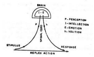
Reaction time of a driver is the time taken by a driver to respond to a situation and it is the sum of lag distance and brake distance. Lag distance is the distance travelled by the vehicle during the time taken by brain of a driver to understand a situation and brake distance is the distance travelled by the vehicle during the response time of the driver.
