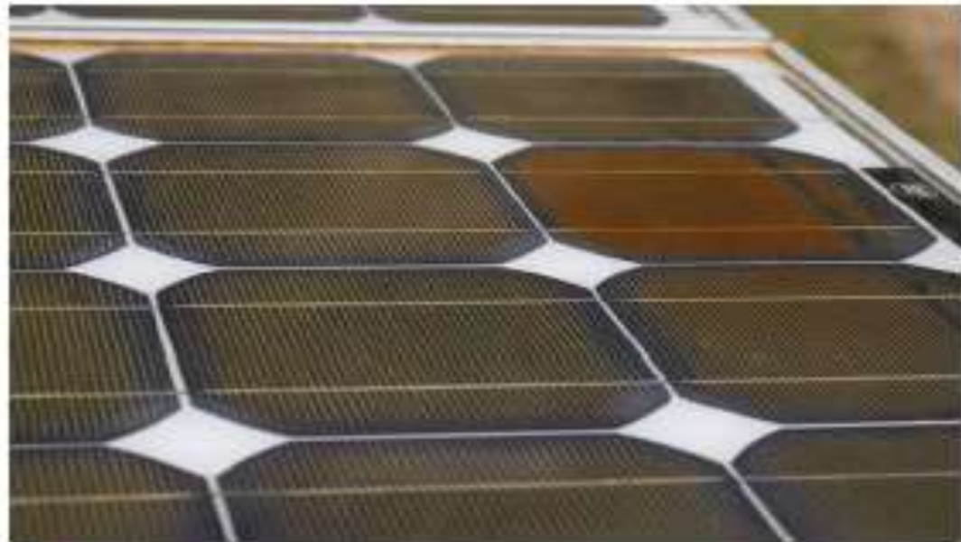
Figure 4.23 The discoloured cell in this array was caused by hot spot heating
